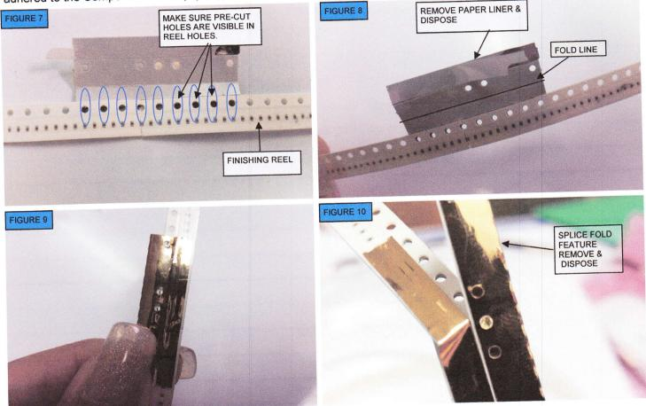
10. Firmly press tape to Component Carrier.
